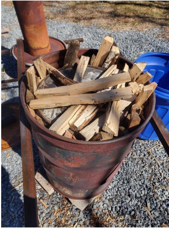
TLUD with top removed to show retort inside
